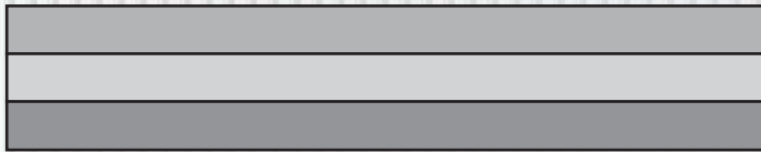
MaxWhite FG Screen Material, Multi-Layer, Cross-Array Coated with Matte White Optical Material. It is flame and mildew resistant.
